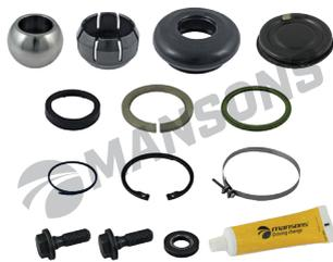
**900.1044** TORQUE ROD REPAIR KIT
