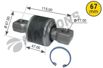
**100.051** TORQUE ROD REPAIR KIT
